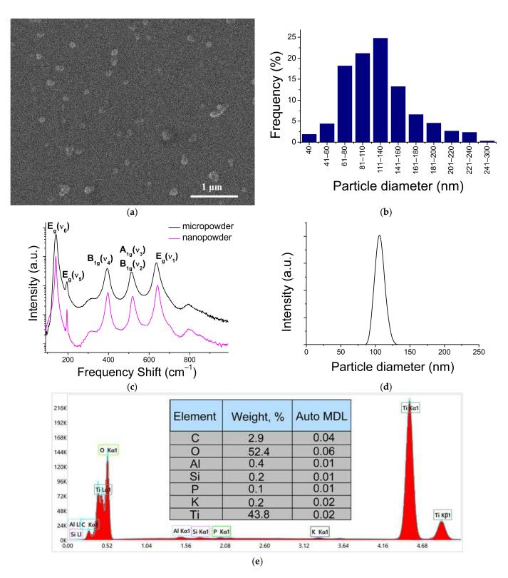
**Figure 1.** Characteristics of the  $TiO_2$  nanofraction: (**a**)  $TiO_2$  nanofraction SEM image; (**b**)  $TiO_2$  NPs' size distribution obtained using SEM data; (**c**) Raman spectra of nano- and microfraction of the E171 powder; (**d**) NPs' size distribution obtained using DLS measurements; (**e**) typical EDX spectrum of the TiO<sub>2</sub> nanofraction of EDX data.
