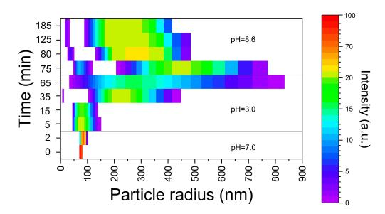
**Figure 3.** Transformation of TiO<sub>2</sub> NPs' size in conditions of sequential passing through GIT section (using DLS data).
