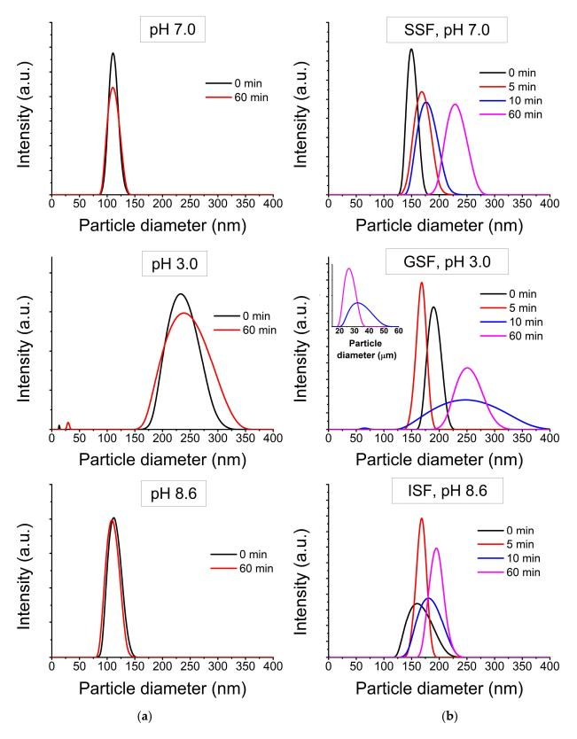
**Figure 2.** Transformation of  $TiO_2$  NPs' size (**a**) in deionized water at various pH values; (**b**) in GIT simulation liquids.
