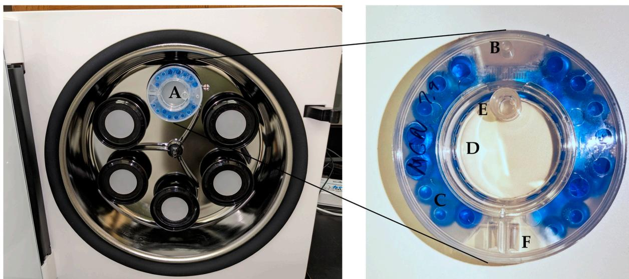
**Figure 6.** ClinoStar<sup>®</sup> incubator and ClinoReactor<sup>®</sup>. (A) Holds up to 6 ClinoReactor<sup>®</sup> bioreactors. (B) Is the port for the sterile water to hydrate the (C). Water beads that create a humidification system. The water beads are separated by a semi-permeable membrane from the (D). Growth culture system, which can be accessed from the (E). Front and (F). Top ports.
