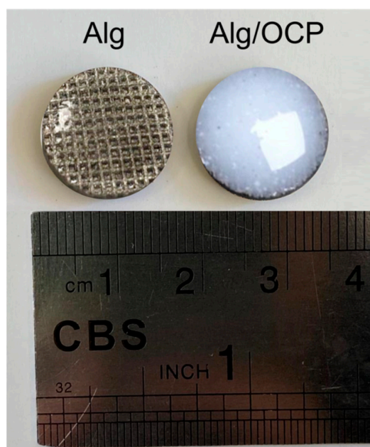
Figure S4. Camera image of the different hydrogel coatings on 3D-printed Ti Gr23 layers.
