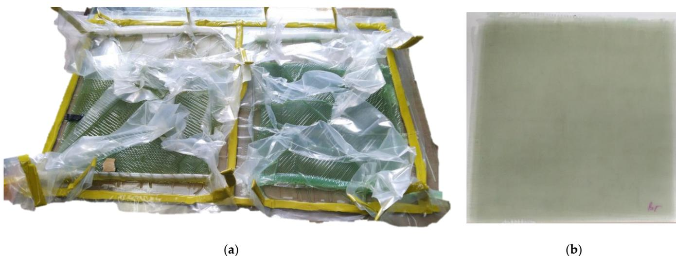
**Figure 5.** Photo: (a) VaRTM of the FGRP sample; (b) cured FGRP sample.
