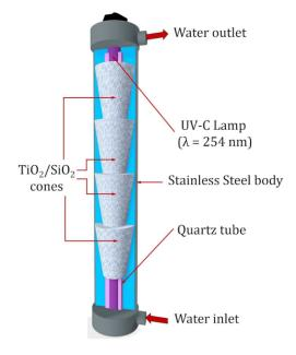
**Figure 9.** Components of the reactor used in the degradation of MTX by photolysis. Interior stainlesssteel cones with the  $TiO_2/SiO_2$  mesh were removed for photolysis experiments.
