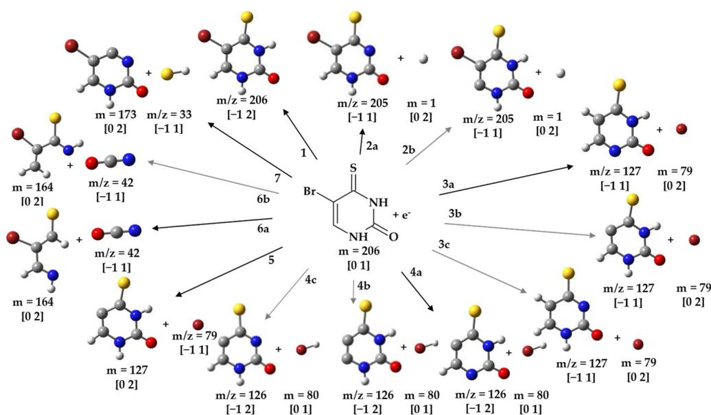
**Figure 2.** Possible DEA-induced reaction pathways for the degradation of BrSU;  $m/z$ , charge, and multiplicity (in the square brackets) are displayed near the particular structures. Thick arrows indicate the most abundant processes observed in the crossed electron–molecular beam experiment.
