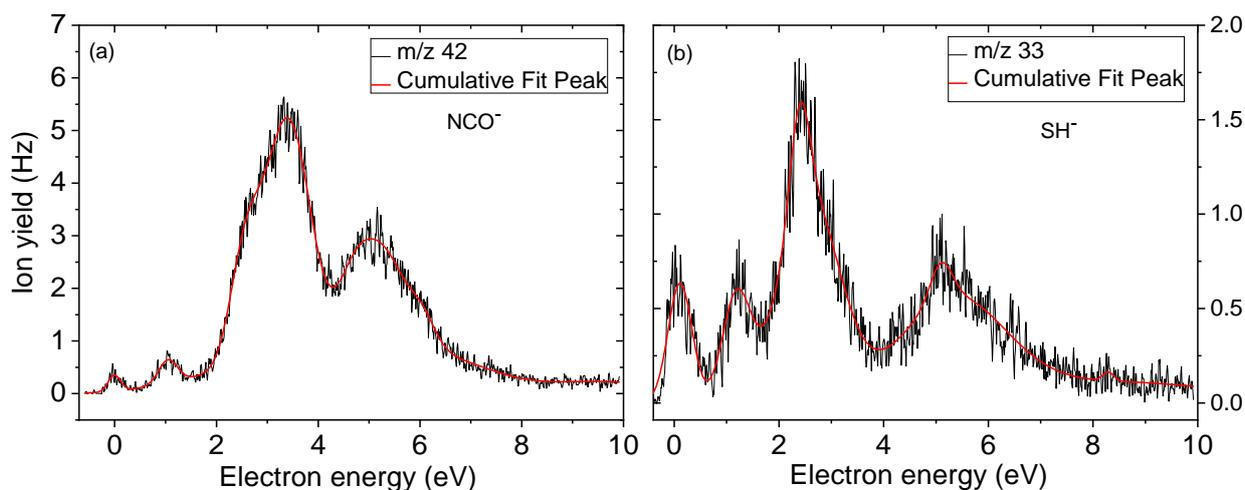
**Figure 4.** Anion efficiency curve for the fragment anions (a)  $\text{NCO}^-$ , and (b)  $\text{SH}^-$  formed upon electron attachment to BrSU.
