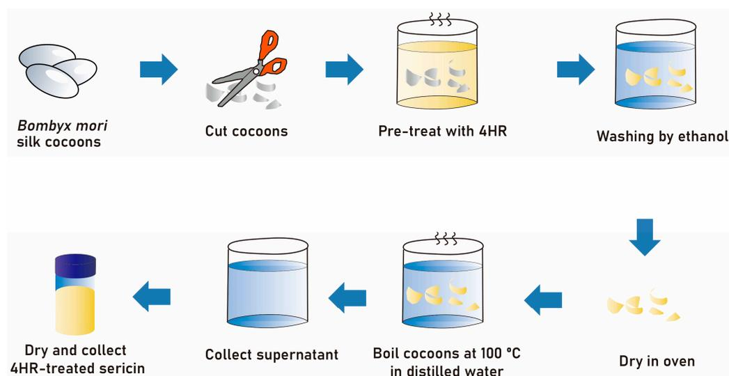
**Figure 6.** Schematic drawing of the method used for 4HR pretreatment of silk cocoons and subsequent extraction of silk sericin.
