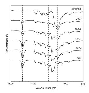
Figure 2. FT-IR spectra of CUC1-CUC4 pentablock copolymers, PCL, and EPE(F38).
