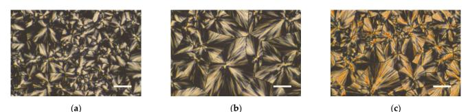
Figure 8. PLOM micrographs of (a) CUC2, (b) CUC3, and (c) CUC4 crystallized at 35 °C. Scale bar is 50 µm.
