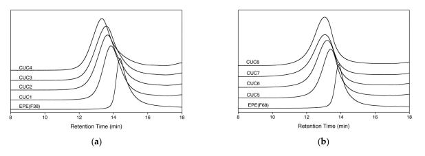
**Figure 1.** SEC chromatograms of CUC copolymers compared with respective macro-initiator EPE. (**a**) CUC1–CUC4 and (**b**) CUC5–CUC8 series.
