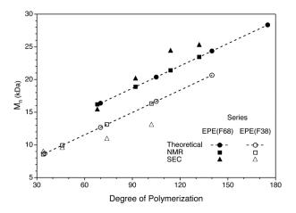
**Figure 4.** Dependence of  $\overline{M}_{n_{CUC}}$  with degree of polymerization.
