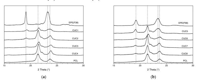
**Figure 6.** WAXD patterns of CUC copolymers compared with respective macro-initiator EPE and PCL. (**a**) CUC1–CUC4 and (**b**) CUC5–CUC8 series.
