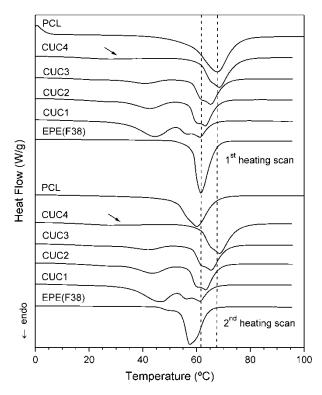
**Figure 5.** First and second heating DSC traces of pentablock CUC1–CUC4 copolymers compared with EPE(F38) and PCL.
