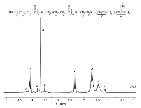
Figure 3. <sup>1</sup>H-NMR spectrum of CUC4 pentablock copolymer.
