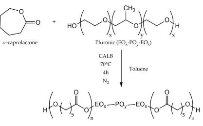
**Scheme 1.** CALB catalyzed ring-opening polymerization of  $\varepsilon$ -CL by using EPE as a macro-initiator.
