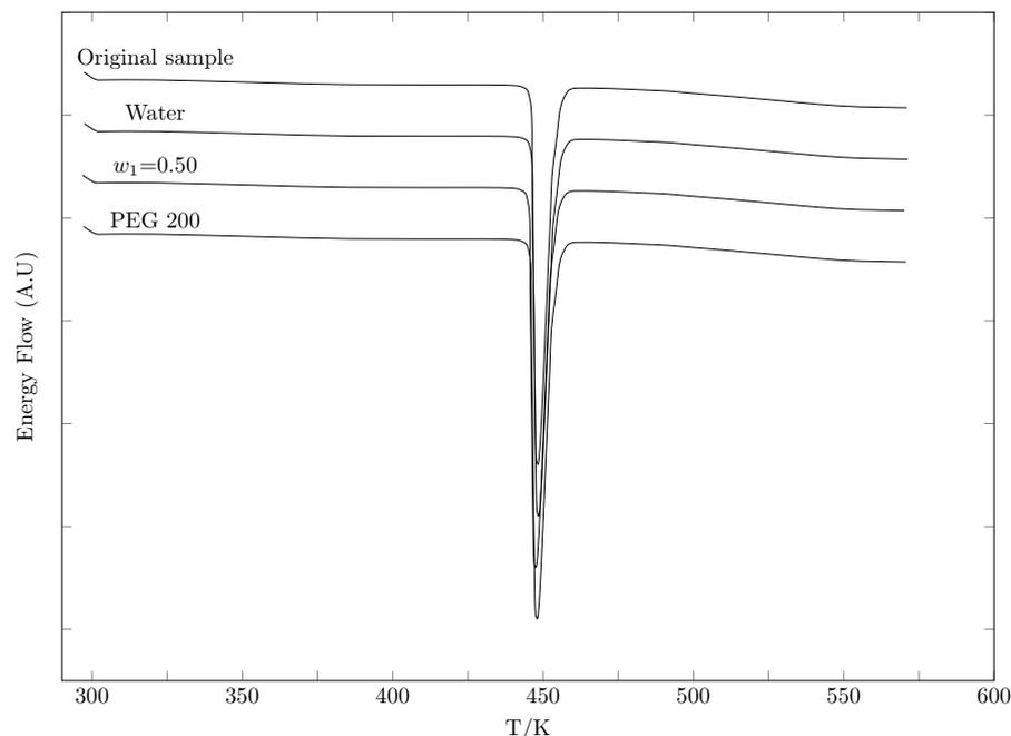
Figure 5. DSC Spectra of Isoniazid.
