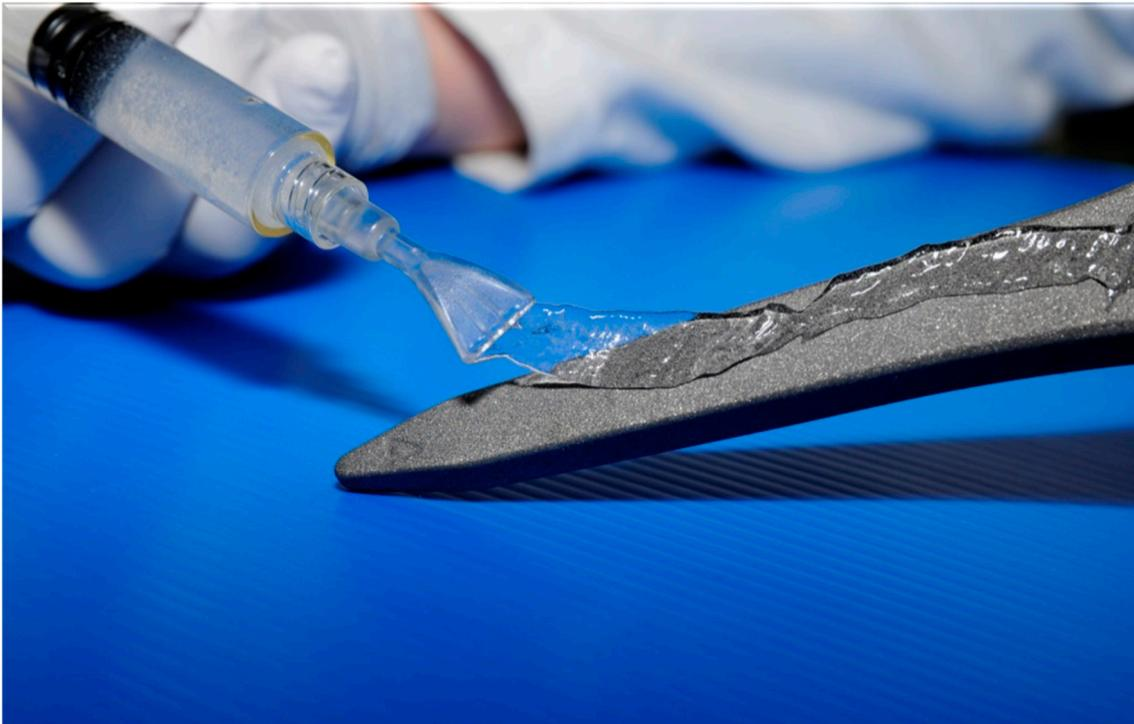
**Figure 6.** Defensive anti-bacterial coating (DAC; Novagenit, Trento, Italy)—a bioabsorbable, antibiotic-containing hydrogel which is designed to slow or prevent bacterial adhesion and biofilm formation.
