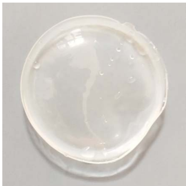
Figure 9. The polymer membrane with 20 wt.% of 2,6-bis(4-methoxybenzoyl)-diaminopyridine before the membrane extraction process.
