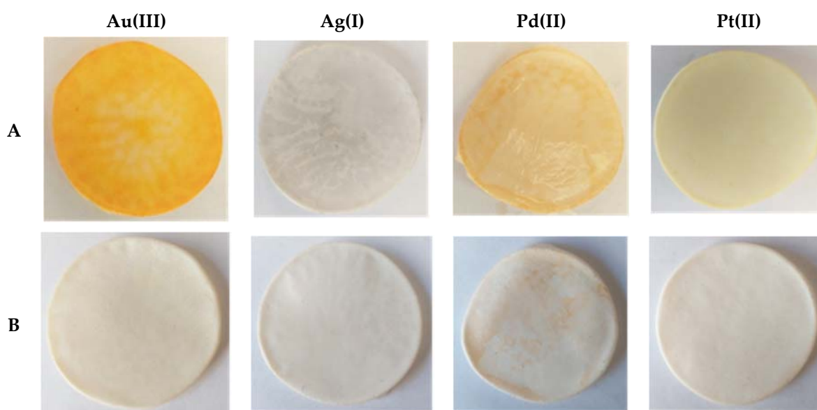
Figure 7. The polymer inclusion membranes containing 2,6-bis(4-methoxybenzoyl)-diaminopyridine after processes: membrane extraction (A), membrane back-extraction (B).
