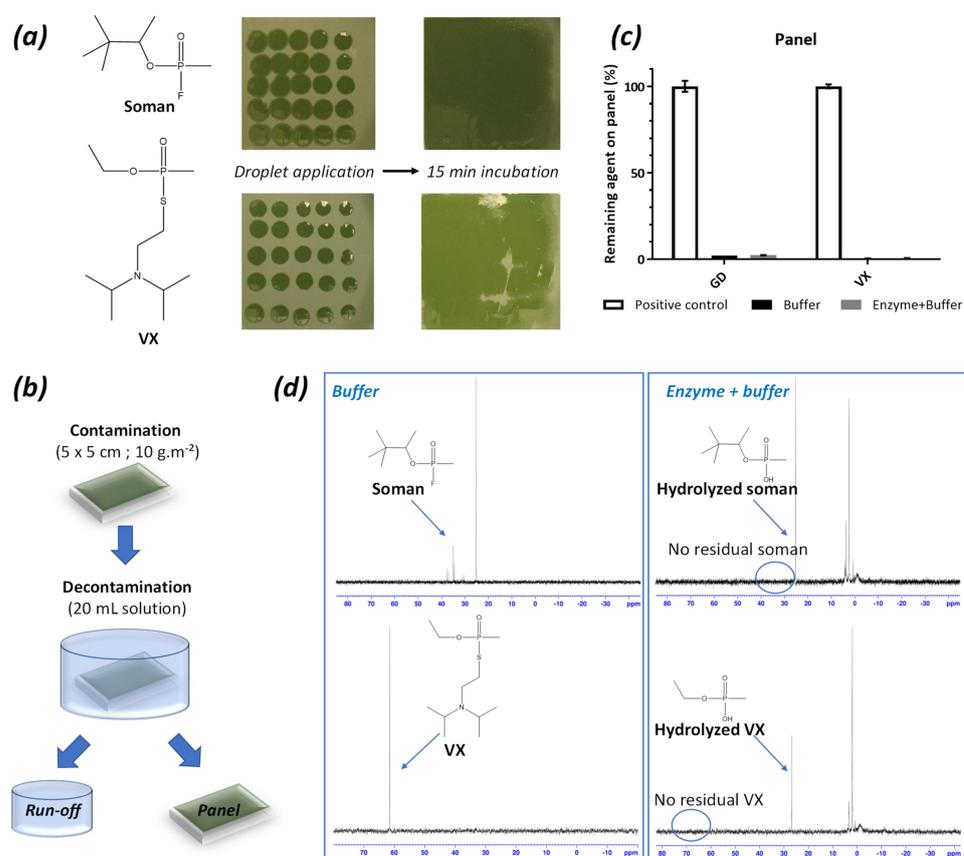
**Figure 4.** Enzyme decontamination of painted panels. (a) Contamination of panels with droplets of agent to reach a final contamination of  $10 \text{ g}\cdot\text{m}^{-2}$  of soman or VX. (b) Contaminated panels ( $5 \times 5 \text{ cm}$ ) are incubated for 15 min in 20 mL of decontamination solutions. (c) Evaluation of residual soman (GD) and VX on panels after decontamination. (d) Evaluating remaining soman and VX in liquid decontamination (run-off) solution.
