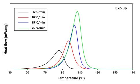
Figure 2. DSC thermograms of epoxy/thiol/MI system obtained at various heating rates.
