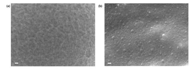
**Figure 7.** FESEM images of the fractured surface of (**a**) NC-3 and (**b**) NC-4 after a notched Izod impact test. A scale bar represents 100 nm.
