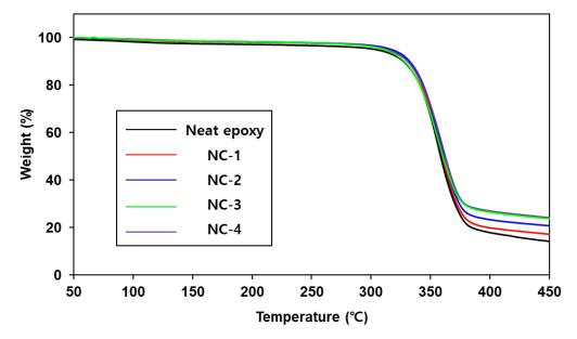
Figure 8. TGA thermograms of neat epoxy and nanocomposites.
