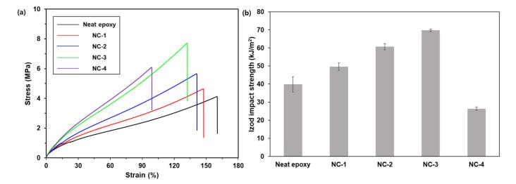
Figure 6. (a) Stress-strain curves of neat epoxy and nanocomposites and (b) Izod impact strength of nanocomposites.
