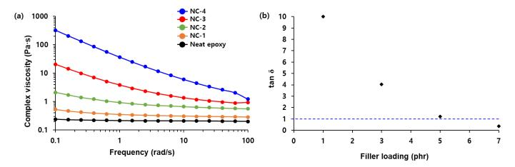
**Figure 5.** (a) Shear-rate dependency of the complex viscosity of neat epoxy and the fumed silica composites and (b) the filler loading dependence of tan  $\delta$  measured at 1 rad/s.
