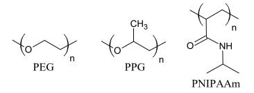
**Figure 2.** Molecular structure of poly(ethylene glycol) (PEG), poly(propylene glycol) (PPG), and poly(*N*-isopropylacrylamide) (PNIPAAm).
