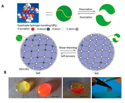
**Figure 10.** (**A**) Scheme of the experimental strategy for obtaining a DEX-UPy hydrogel with shearthinning and self-integration properties; (**B**) visualization of these properties (scale bar corresponds to 5 mm). Reprint with permission [152]; Copyright 2015, Wiley.
