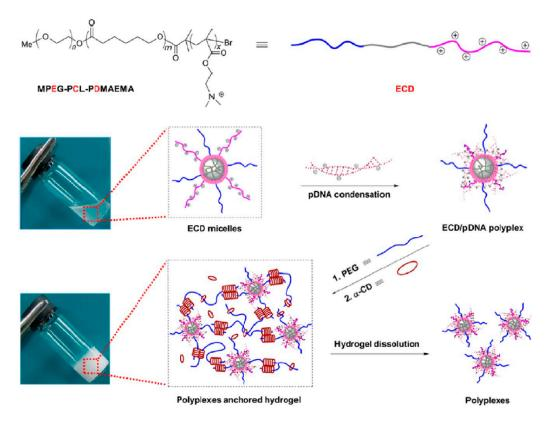
**Figure 9.** Schematic illustration for obtaining ECD/pDNA anchored  $\alpha$ -CD/PEG supramolecular hydrogels (ECD corresponds to the MPEG-PCL-PDMAEMA, where E: MPEG, C: PCL, and D: PDMAEMA). Reprint with permission [142]; Copyright 2012, American Chemical Society.
