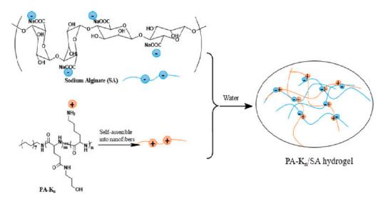
**Figure 8.** Cationic peptide amphiphiles-based supramolecular hydrogels with sodium alginate (n—the quantity of lysine unit in the peptide segment). Reprint with permission [127]; Copyright 2017, American Chemical Society.
