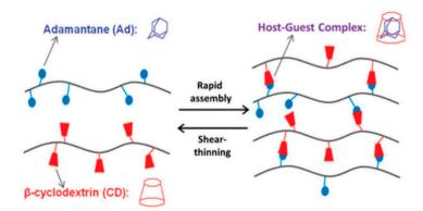
**Figure 5.** The host–guest interaction between  $\beta$ -cyclodextrin and adamantine. Reprint with permission [36]; Copyright 2019, Wiley.
