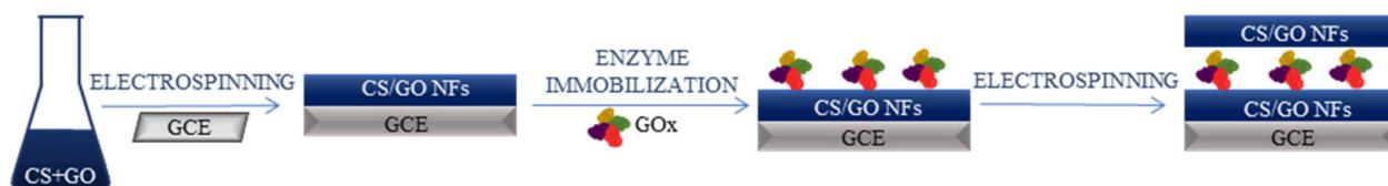
**Figure 8.** Schematic process of the synthesis of GOx/CS/GO nanofibers [45]; CS—chitosan, GO—graphene oxide, GCE—glassy carbon electrode, GOx—glucose oxidase.
