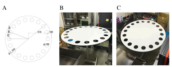
**Fig. S1.** Blueprint used to cut out from an acrylic sheet (A). A view of the Barnes maze set up at the site of the experiment. There are some spatial recognition clues for rats around the Barnes maze (B, C).
