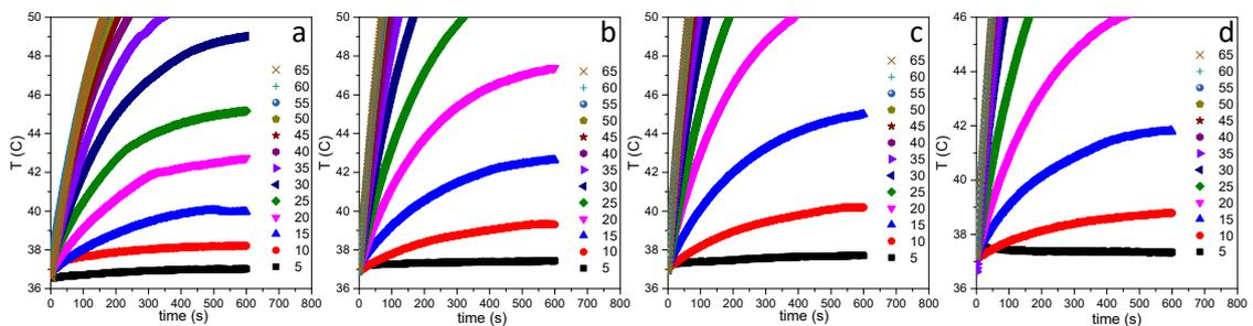
Figure S7. Heating curves of  $Zn_xFe_{3-x}O_4$  MNPs with (a)  $x = 0$ , (b)  $x \sim 0.1$ , (c)  $x \sim 0.3$  and (d)  $x \sim 0.5$  dispersed in water at a concentration of 1 mg/mL, recorded as a function of AC magnetic field amplitudes at 355 kHz.
