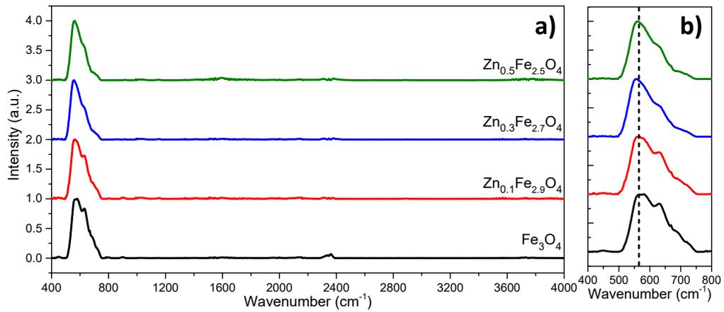
**Figure S3.** (a) FT-IR spectra of uncoated  $Zn_xFe_{3-x}O_4$  MNPs ( $0 \leq x < 0.5$ ) and (b) Zoom in the 400–800  $cm^{-1}$  region of FT-IR spectra. The spectra are normalized to the highest absorption band and shifted for clarity.
