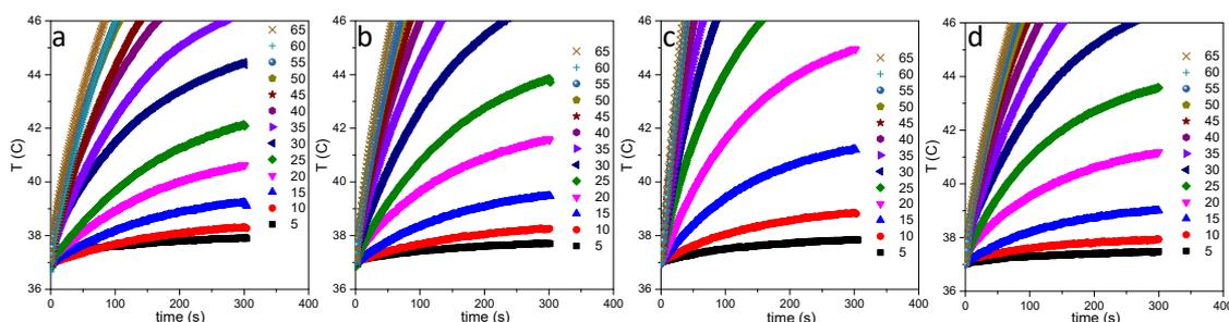
**Figure S9.** Heating curves of  $Zn_xFe_{3-x}O_4$  MNPs with (a)  $x = 0$ , (b)  $x \sim 0.1$ , (c)  $x \sim 0.3$  and (d)  $x \sim 0.5$  randomly dispersed in PEG 8k at a concentration of 1 mg/mL, recorded as a function of AC magnetic field amplitudes at 355 kHz.
