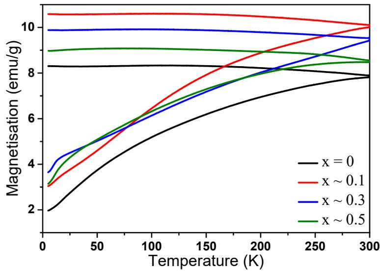
Figure S5. ZFC and FC magnetization curves of  $Zn_xFe_{3-x}O_4$  MNPs ( $0 \leq x < 5$ ).
