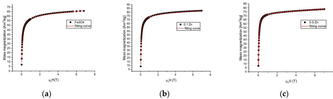
Figure S6. Magnetization curve fitting for the  $Zn_xFe_{3-x}O_4$  MNPs with  $x = 0$  (a),  $x \sim 0.1$  (b) and  $x \sim 0.5$  (c) at 300 K, the black squares represent the experimental data and the red lines are the fitting curves.
