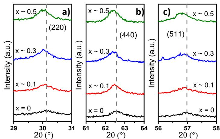
**Figure S1.** Zooms on the (220) (a), (511) (b) and (440) (c) diffraction peak regions of XRD diffraction patterns of Zn<sub>x</sub>Fe<sub>3-x</sub>O<sub>4</sub> MNPs with different zinc doping level ( $0 \leq x < 0.5$ ).
