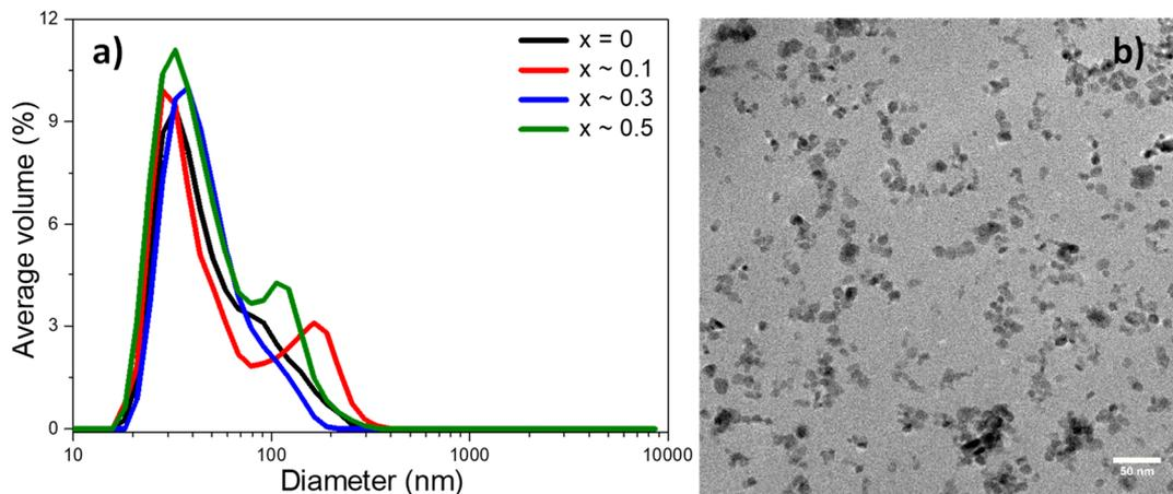
**Figure S4.** (a) DLS size distribution plots of uncoated  $Zn_xFe_{3-x}O_4$  MNPs ( $0 \leq x < 0.5$ ) and (b) TEM image of the particles. The spectra are normalized to the highest absorption band and shifted for clarity.
