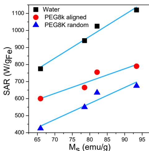
**Figure S8.** The saturation SAR values of four types of MNPs in both media as a function of the magnetization saturation of MNPs. The blue lines represent linear fits.
