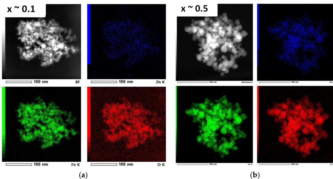
**Figure S2.** TEM image of Zn<sub>x</sub>Fe<sub>3-x</sub>O<sub>4</sub> MNPs with x ~ 0.1 (a) and x ~ 0.5 (b) and the corresponding EDX mapped images for Zinc (blue), Iron (green) and Oxygen (red).
