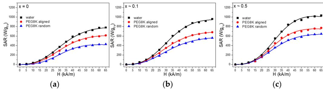
**Figure S12.** Fitting the experimental SAR data (dots) of the samples with  $x = 0$  (a),  $x \sim 0.1$  (b) and  $x \sim 0.5$  (c) with a fitting function (lines) given by equation 12 from the main text, which takes into account the dependence of both Neel and Brown relaxation times on the AMF amplitude.
