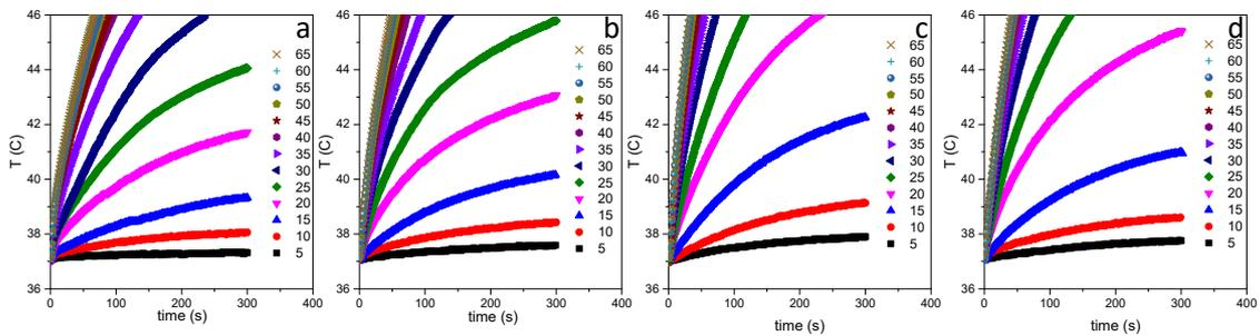
**Figure S11.** Heating curves of  $Zn_xFe_{3-x}O_4$  MNPs with (a)  $x = 0$ , (b)  $x \sim 0.1$ , (c)  $x \sim 0.3$  and (d)  $x \sim 0.5$  pre-aligned in a static magnetic field of 15 mT while being dispersed in PEG 8k at a concentration of 1 mg/mL, recorded as a function of AC magnetic field amplitudes at 355 kHz.
