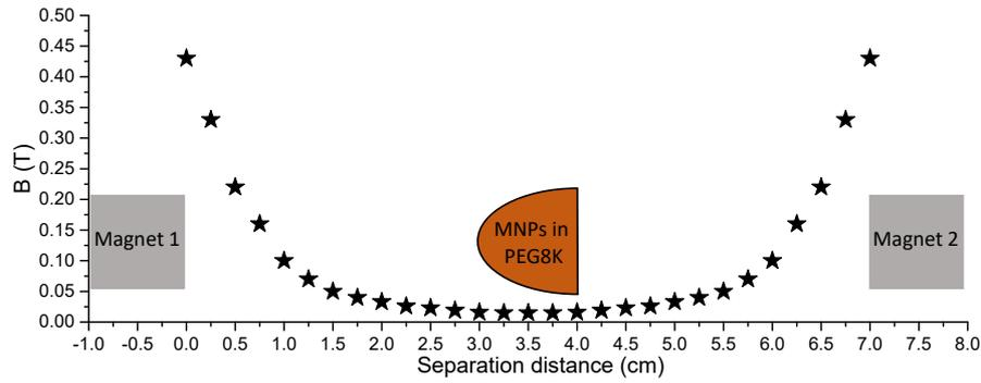
**Figure S10.** Magnetic induction calibration curve between two neodymium (Ne-Fe-B) magnets separated by 7 cm one from the other.
