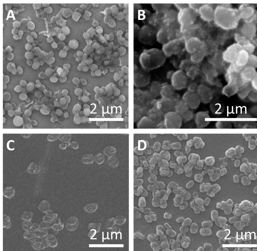
**Figure 2.** Characterization of submicrometric capsules. Representative SEM images of (A) SiO<sub>2</sub> capsules with low amount of tetraethyl orthosilicate (TEOS), (B) SiO<sub>2</sub> capsules with high amount of TEOS, (C) (DEXS/PARG)<sub>4</sub> capsules, and (D) (PSS/PAH)<sub>4</sub> capsules.
