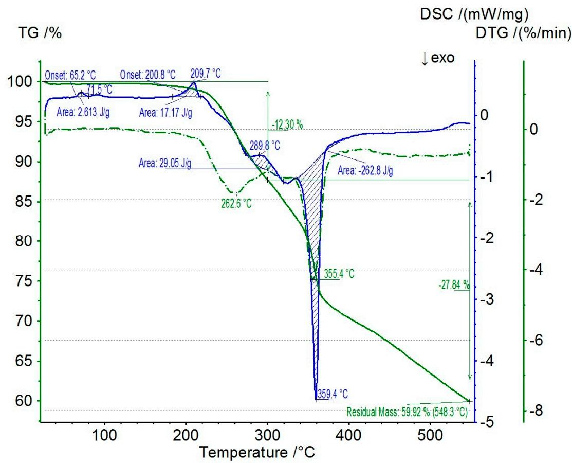
Fig. S8. TG/DTG-DSC curves of compound **2b**.
