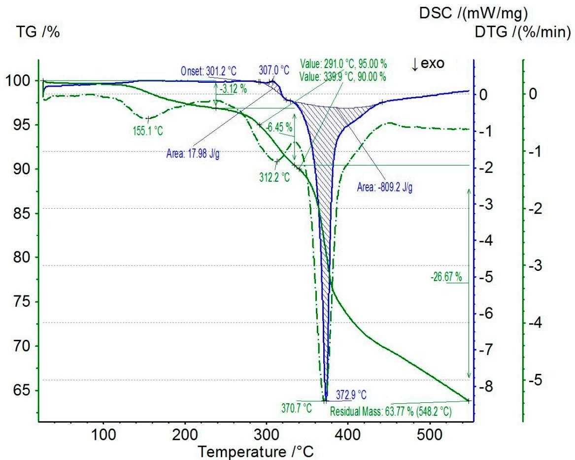
Fig. S38. TG/DTG-DSC/dDSC curves of compound 4.
