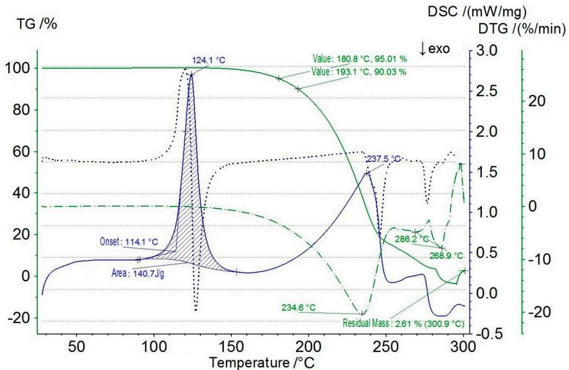
Fig. S39. TG/DTG-DSC/dDSC curves of compound 9.
