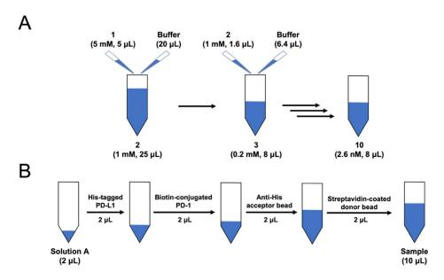
Figure S5. Preparation of (A) sample dilutions and (B) reaction samples.
