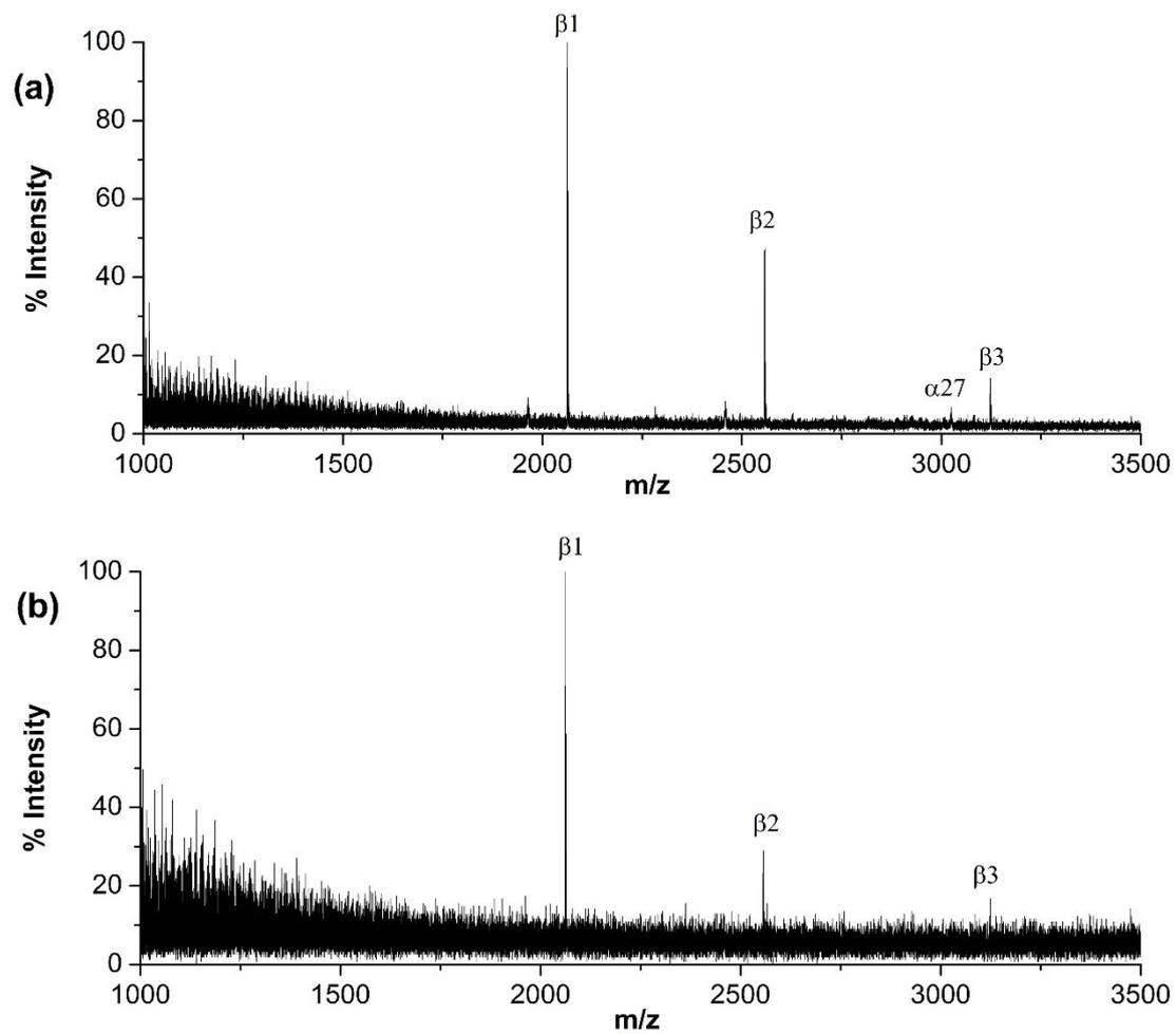
Fig. S2 MALDI mass spectra of tryptic digests of  $\beta$ -casein after enrichment using QB. The amounts of tryptic digest of  $\beta$ -casein used in the experiments were (a) 300 fmol and (b) 30 fmol.
