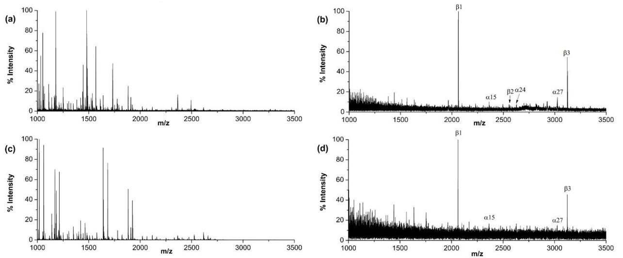
Fig. S1 MALDI mass spectra of the tryptic digest mixtures of  $\beta$ -casein and BSA (a, c) without or (b, d) with enrichment. The molar ratios of  $\beta$ -casein to BSA were (a, b) 1:10 and (c, d) 1:100, respectively. The concentration of  $\beta$ -casein was 3 pmol.
