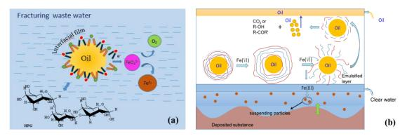
**Figure 6.** The possible mechanism of the oxidation process, showing (**a**) demulsification and (**b**) visbreaking.
