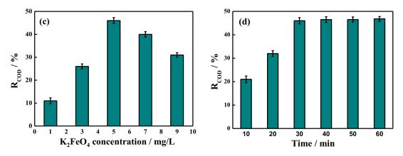
**Figure 4.** COD removal rate by potassium ferrate oxidation under different conditions of (**a**) pH value, (**b**) temperature, (**c**) the addition of potassium ferrate, and (**d**) reaction time.
