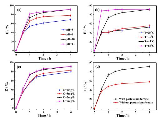
**Figure 1.** Demulsification efficiency of potassium ferrate under different conditions of (**a**) pH value, (**b**) temperature, (**c**), the addition of potassium ferrate, and (**d**) presence and absence of potassium ferrate.
