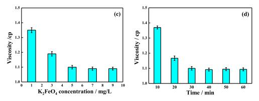
**Figure 3.** Visbreaking by potassium ferrate oxidation under different conditions of (**a**) pH value, (**b**) temperature, (**c**) the addition of potassium ferrate, and (**d**) reaction time.
