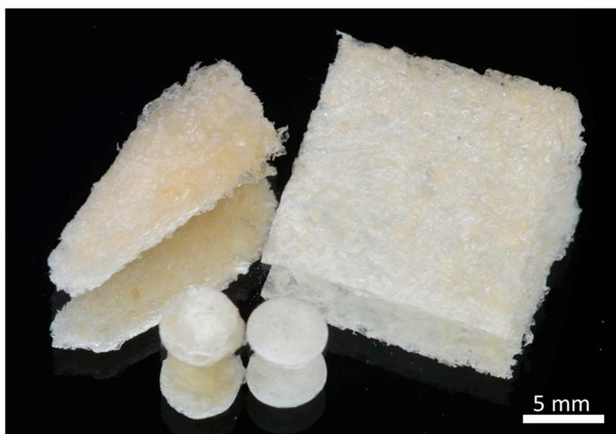
**Figure 6.** The fabricated CS-DA scaffold after freeze-drying.
