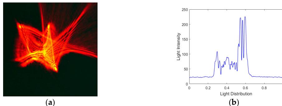
**Figure 7.** (a) The image captured by CCD with random aberration generated by the MFDM; (b) light intensity distribution.
