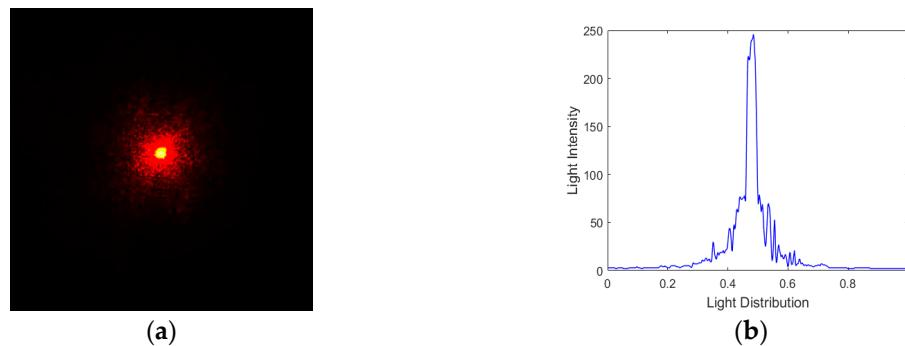
**Figure 5.** (a) The focal spot image captured by Charge-coupled Device (CCD) without aberration disturbance; (b) light intensity distribution
