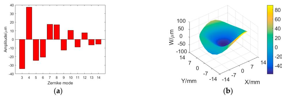
**Figure 6.** Target aberration. (a) Zernike mode numbers of the target aberration; (b) the aberration wavefront.
