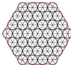
**Figure 2.** The arrangement of electromagnetic actuators of magnetic fluid deformable mirror (MFDM).
