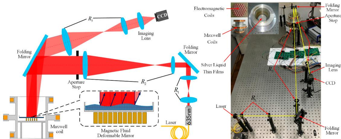
**Figure 4.** The schematic and actual layout of the experimental setup of wavefront sensorless (WFSless) adaptive optics (AO) system.
