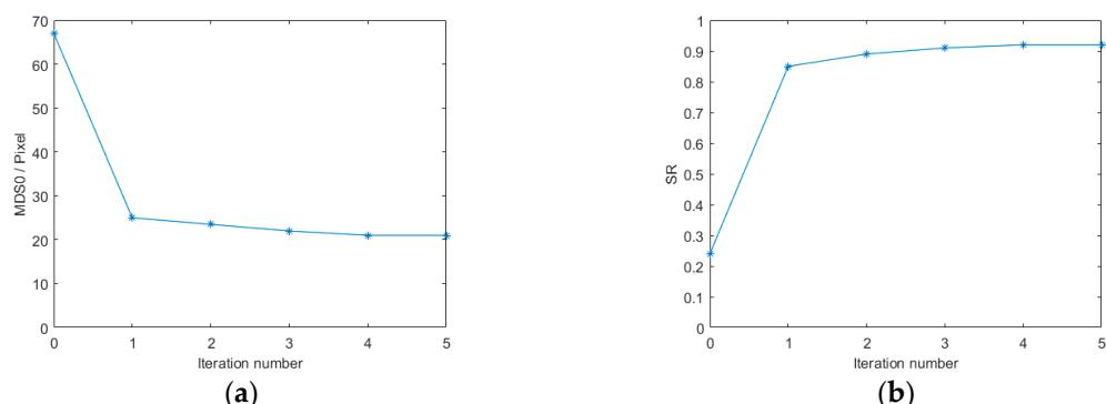
**Figure 9.** The trend of the performance metric (a)  $MDS_0$  curve; (b) Sterhl ratio (SR) curve.
