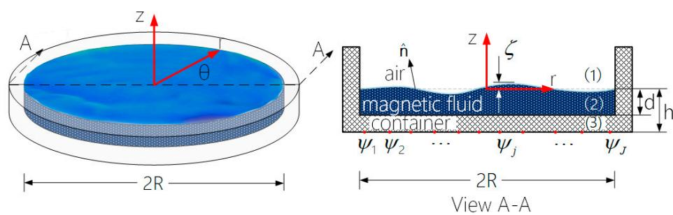
**Figure 1.** Geometric representation of a circular magnetic fluid deformable mirror.
