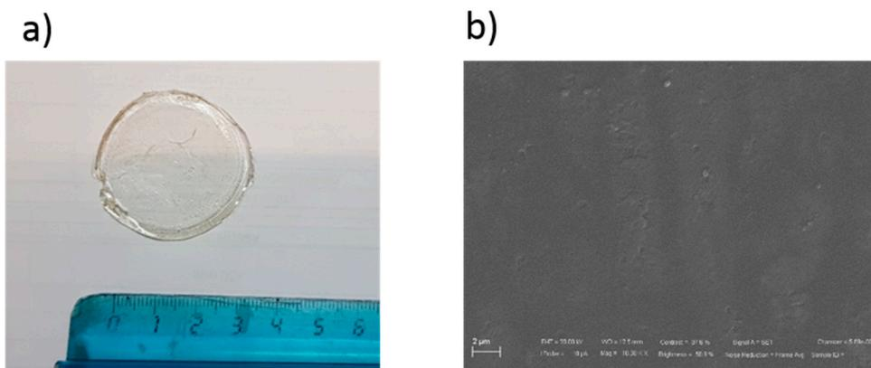
**Figure 1.** Image (a) and SEM picture (b) of a typical film obtained by copolymerization of acryloyloxyundecyltriethylammonium bromide (AUTEAB) with 2-hydroethyl methacrylate (HEMA).
