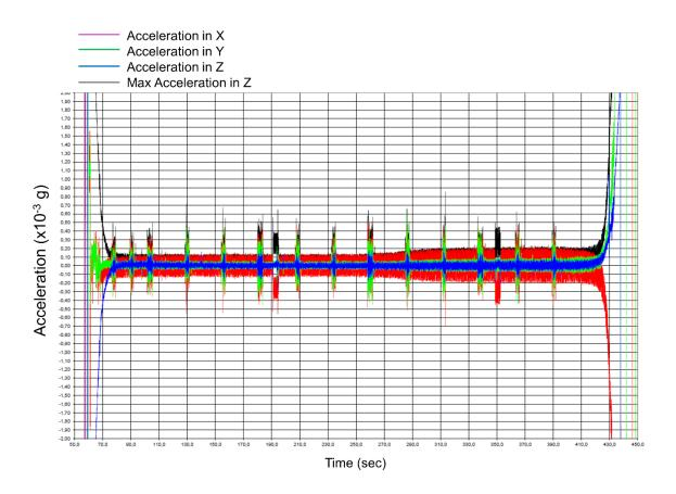
Figure S1. Gravity profile of the TEXUS-54 flight. Recording provided by OHB System AG.
