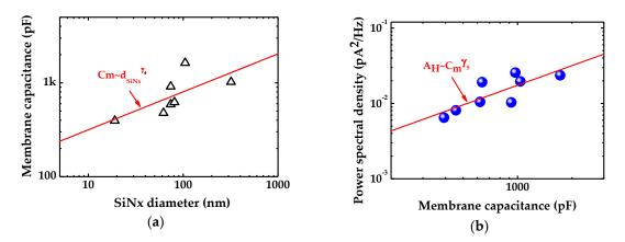
**Figure 6.** Impact of graphene suspended area on noise in high-frequency region: (a) Membrane capacitance measured by membrane test in 2 M KCl solution versus underlying  $SiN_x$  diameter; and (b) the relationship between high-frequency noise and membrane capacitance. The fit line determines a dependency of high-frequency noise on membrane capacitance.
