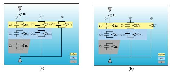
**Figure 7.** Equivalent circuit of monolayer graphene nanopore regime: (**a**) equivalent circuit of the extensive suspended model; and (**b**) the equivalent circuit of the narrow free-standing model.
