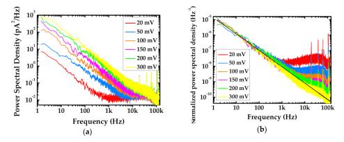
**Figure 2.** Noise traces of a graphene nanopore with diameter of 5 nm at 100 mM KCl: (**a**) Noise power spectral density at varied bias voltage; and (**b**) normalized noise power spectral densities. The black straight line represents the average result of the low-frequency linear fitting.
