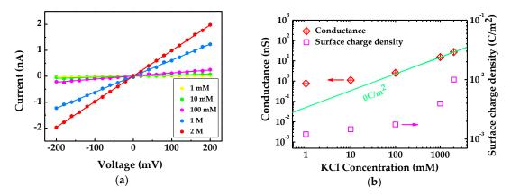
**Figure 8.** (a) *I-V* curve of a graphene nanopore with a diameter of 1.2 nm; and (b) the conductance and surface charge density against concentration of KCl. The green line shows the fitting without contribution of surface charge distribution.
