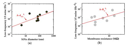
**Figure 4.** (a) Low-frequency noise power plotted against the underlying  $SiN_x$  diameter. The yellow number in the center of the points represent the pore size of each graphene nanopore; and (b) the noise in the low-frequency range versus membrane resistance. The red solid line fits to the resistance of eight graphene nanopores.
