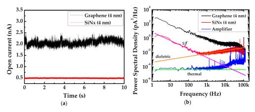
**Figure 1.** Comparison of noise level in different material nanopore systems measured at 1 M KCl and 100 mV: (a) Open current of two comparable nanopores punched on graphene and SiN<sub>x</sub>, respectively; and (b) noise power spectral densities of the two nanopores. The fitting executed according to the noise polynomial  $S = Af^{-\beta} + B + Cf + Df^2$  is shown for the SiN<sub>x</sub>-based nanopore sensor.
