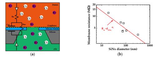
**Figure 5.** (a) Schematic of free-standing monolayer graphene nanopore and equivalent circuit of the system; and (b) the membrane resistance as a function of underlying  $SiN_x$  diameter.
