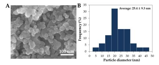
**Figure 1.** (**A**) Scanning electron microscopic (SEM) images and (**B**) size distribution of ZnO NPs. Particle size distribution was determined by randomly selecting 200 particles from the SEM images.
