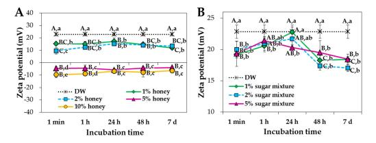
**Figure 3.** Zeta potentials of ZnO NPs in different concentrations of (**A**) honey and (**B**) sugar mixtures. Different capital letters (A–C) indicate significant differences between incubation times at the same concentration (p < 0.05). Different lower-case letters (a–e) indicate significant differences between concentrations after the same incubation time (p < 0.05). Sugar mixtures consist of equivalent amounts of fructose, glucose, sucrose and maltose.
