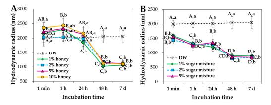
**Figure 2.** Hydrodynamic radii of ZnO NPs in different concentrations of (**A**) honey and (**B**) sugar mixtures. Different capital letters (A–D) indicate significant differences between incubation times at the same concentration (p < 0.05). Different lower-case letters (a,b) indicate significant differences between concentrations after the same incubation time (p < 0.05). Sugar mixtures consist of equivalent amounts of fructose, glucose, sucrose and maltose.
