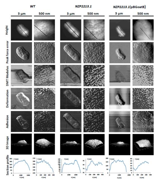
**Figure 4.** Atomic force microscopy (AFM) images of wild-type *Mesorhizobium loti* NZP2213 (WT), the NZP2213.1 mutant, and the complemented NZP2213.1(pBGoatB) strain. The columns show air-dried whole cells ( $3 \times 3 \mu m$ ) and surface ultrastructures at a high resolution ( $500 \times 500 nm$ ). Section profiles, presented in the lower panel, correspond to the height profiles (upper panel) obtained along the black scan lines shown in them.
