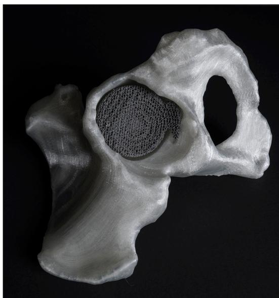
**Figure 1.** A patient-specific implant designed based on computed-tomography (CT) images and AM with selective laser melting. The corresponding bone is also segmented from CT images and AM using fused deposition modeling. Made at Additive Manufacturing Lab, TU Delft (Researchers: Eline Kolken and Saber Amin Yavari).
