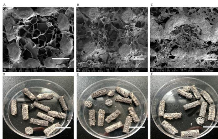
**Figure 2.** Surface characterization and gross view of hybrid scaffolds by scanning electron micrograph (SEM). Gel:nHA = 1:0 group (A,D); Gel:nHA = 1:1 group (B,E); Gel:nHA = 1:3 group (C,F). Scale bar: 500  $\mu\text{m}$  (A–C), 15 mm (D–F).
