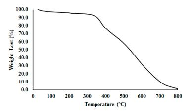
Figure S2. Thermogravimetric analysis of tetrakis(carboxyphenyl) porphyrin (TCPP) molecule.
