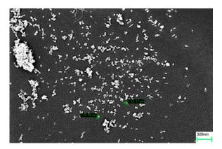
**Figure S1.** Scanning electron microscopy (SEM) image of redox-responsive tetrakis(carboxyphenyl) porphyrin polysilsesquioxane nanoparticles (RR-TCPP-PSilQNPs). Green marks indicate the size of individual nanoparticles. Scale bar = 300 nm.
