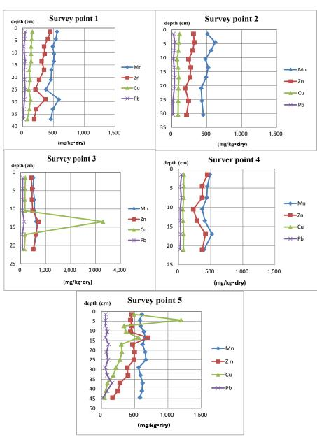
Figure 3. Concentrations of metals in sediment core samples.
