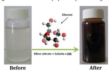
**Figure 1.** Schematic of the preparation process of Ag-NPs.
