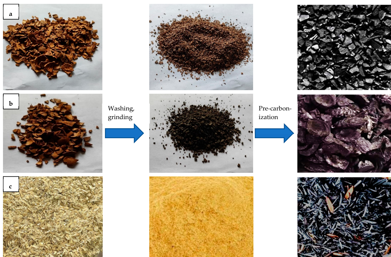
Figure 1. View of biomass after the pre-carbonization process: walnut shell (a), apricot stones (b) and rice husk (c).
