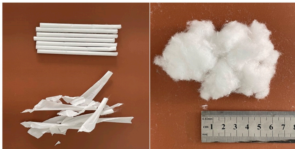
Figure 12. Appearance of acetate fibers.
