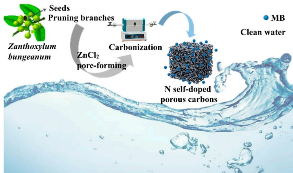
**Figure 1.** Schematic depiction of the synthesis and application of N self-doped porous carbons.
