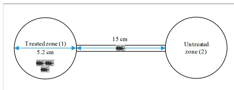
**Figure 7.** Modified tunnel-type device to measure the repellent effect on maize weevils (sketch made by authors).
