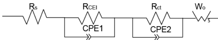
Figure S10. The equivalent circuit models of the EIS fitting.
