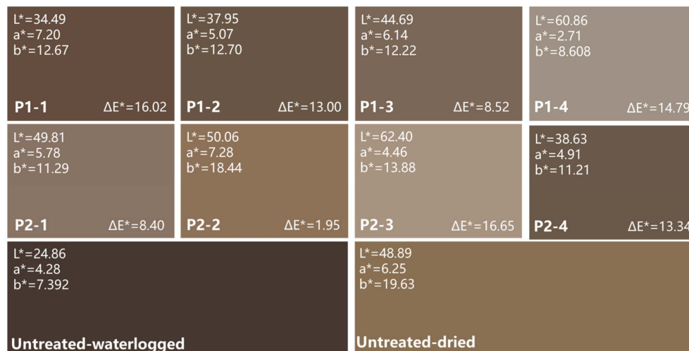
Figure 4. Simulated color according to the CIELab color model of the wood samples.
