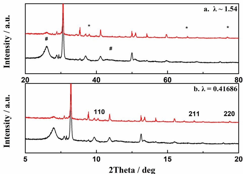
**Figure 4.** X-ray powder diffraction patterns of plasma deposition samples. (a) Diffraction patterns taken with  $\lambda \sim 1.54$  Å, (b) diffraction pattern converted to  $\lambda = 0.41686$  Å, (\*) peaks of cg-N, (#) peaks of CNT.
