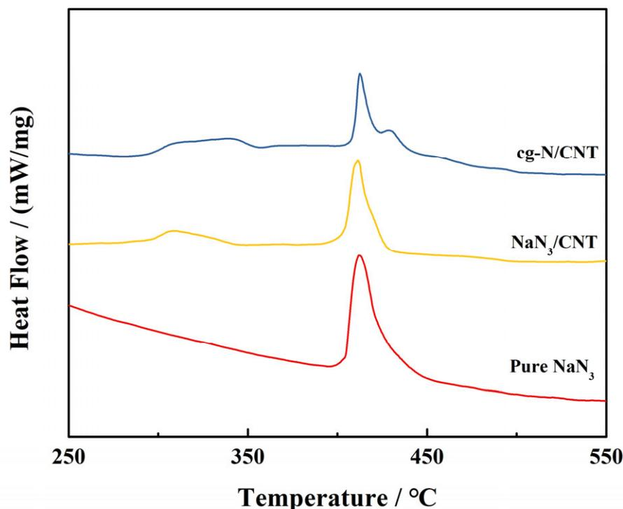
**Figure 6.** DSC curves of pure NaN<sub>3</sub>, NaN<sub>3</sub>/CNT and cg-N/CNT obtained at a heating rate of 10 °C/min.
