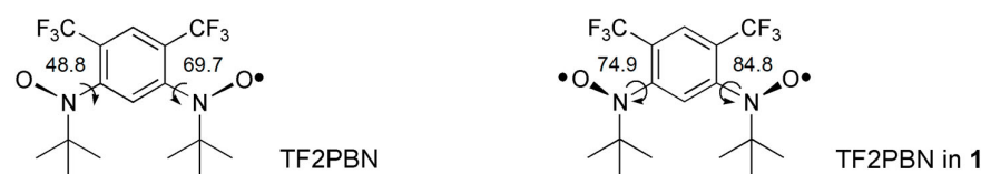
Scheme 2. The torsion angles (left) before and (right) after adduct formation. \theta_1 and \theta_2 are shown.
