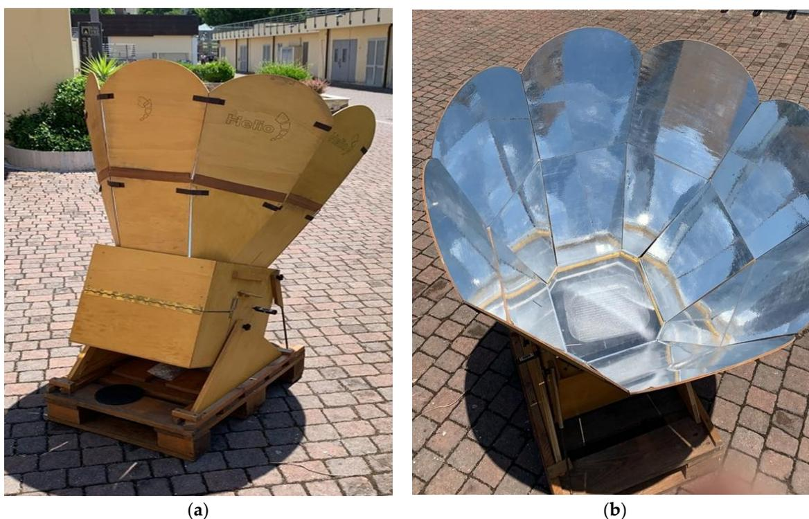
**Figure 1.** Helio© solar cooker, kindly provided by Eng. Alessandro Varesano. (a) Structure of the reflection panels and cooking chamber; (b) Vision of the cooking chamber from the glass panel. The grilling pan is visible inside.
