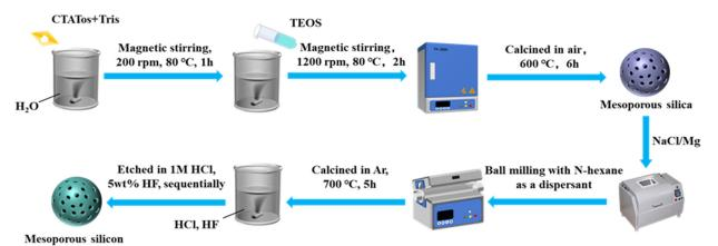
Figure 6. A schematic diagram of the preparation process for M-Si.
