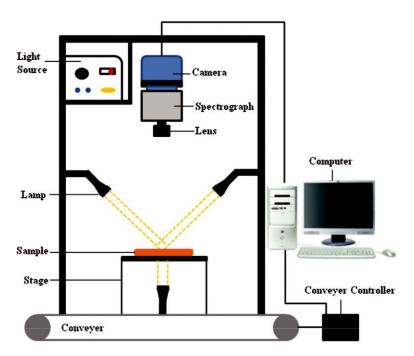
Figure 3. The main components of the HSI system [29].
