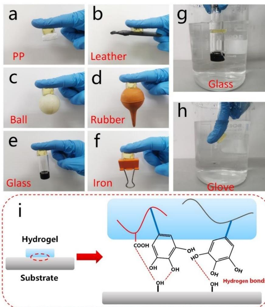
**Figure 6.** Adhesive properties of PGTA organohydrogels. Organohydrogels can be bonded on various surfaces, including (a) PP; (b) leather; (c) ball; (d) rubber; (e) glass; (f) iron; (g,h) self-adhesiveness of the glue to glass and laboratory gloves in water; (i) schematic illustration of the adhesion mechanism of organohydrogels.
