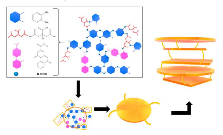
**Figure 7.** Schematic structure of PCDs produced using 1,2-diaminobenze and citric acid. Reprinted with permission from Mintz et al. [109].
