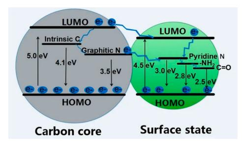
**Figure 4.** Scheme of the fluorescence emission of CQNDs based on different core/shell size ratios and surface residues. Reprinted with permission from Yu et al. [66] under CC BY 4.0.
