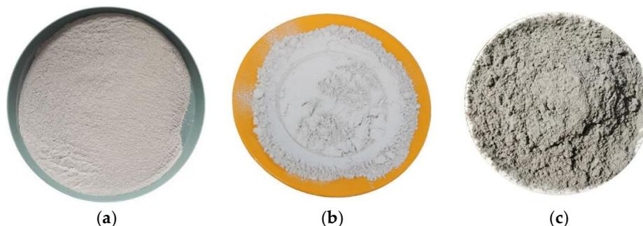
Figure 7. Sample of PC, PG, and GGBS. (a) PG; (b) GGBS; (c) PC.
