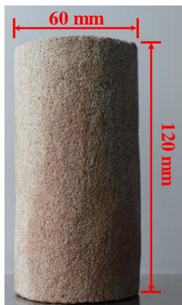
**Figure 13.** Dimensions of Pisha sandstone specimens.
