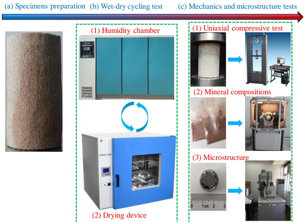
**Figure 14.** Procedure of the wet–dry cycle test.
