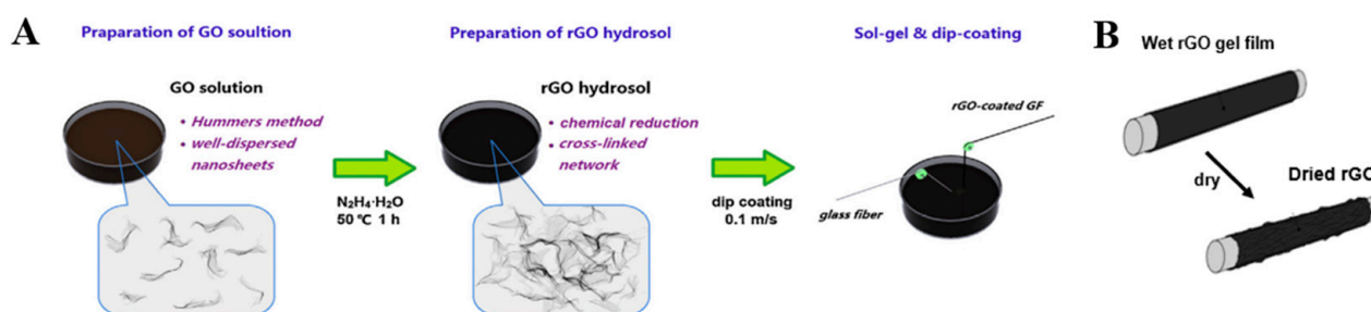
Figure 7. (A) Preparation schematic of graphene-coated GFs through sol-gel and dip-coating techniques. (B) Formation of the wrinkled rGO coatings onto GFs. Reproduced with permission from reference [87]. Copyright 2019 Journal of Materials Science & Technology .
